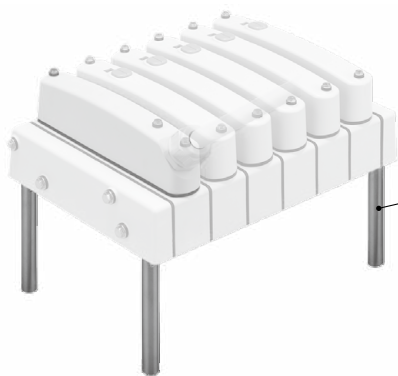
Mounting leg (M6) Tightening torque: 4.9 N·m
